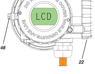
Guide **cable** through cable gland **38** from the bottom; observe especially the shielding.
