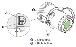
After shifting the key protection cap  $\boldsymbol{A}$ , insert screw driver or pin ( $\mathcal{O}$  < 3 mm) into hole  $\boldsymbol{B}$  and press down to the second pressure point.
