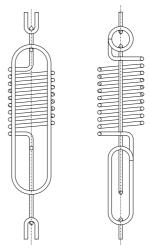
It is hooked onto the suspension chain of the displacer in place of 7 chain links (105 mm). This spring is specially matched to the resonance frequency of the displacer and is made of stainless steel 1.4310 (operating temperature up to 250 °C) or Hastelloy C (operating temperature up to 350 °C).
