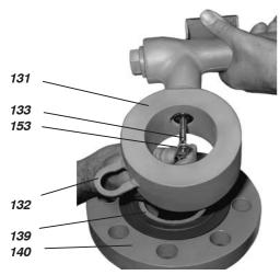
Place the seal *139* <sup>1)</sup> on the connecting flange *140*. Insert displacer in displacer chamber or vessel. Hold 244LD *LevelStar 131* above connecting flange. Engage eyelet *153* of displacer chain in notch in transmission lever *133* and fit wafer body onto connecting flange.
